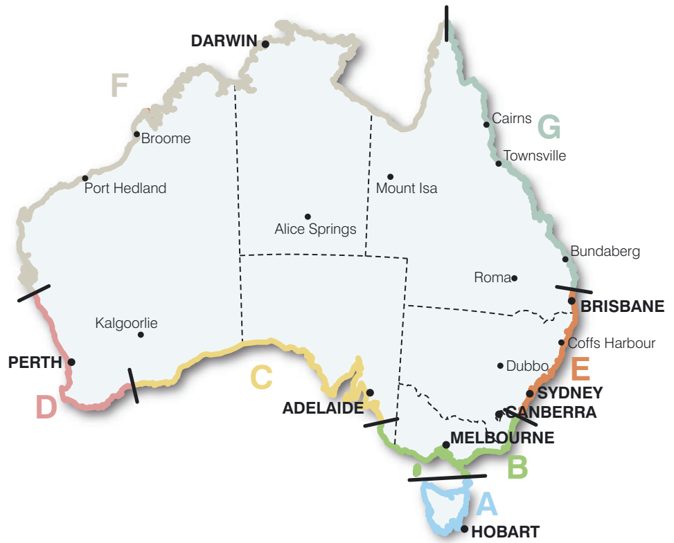
Figure 9.1: Marine borer hazard zones.
