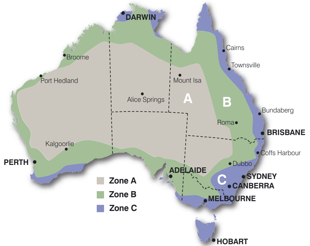
Figure 8.2: Hazard zone for embedded corrosion.
