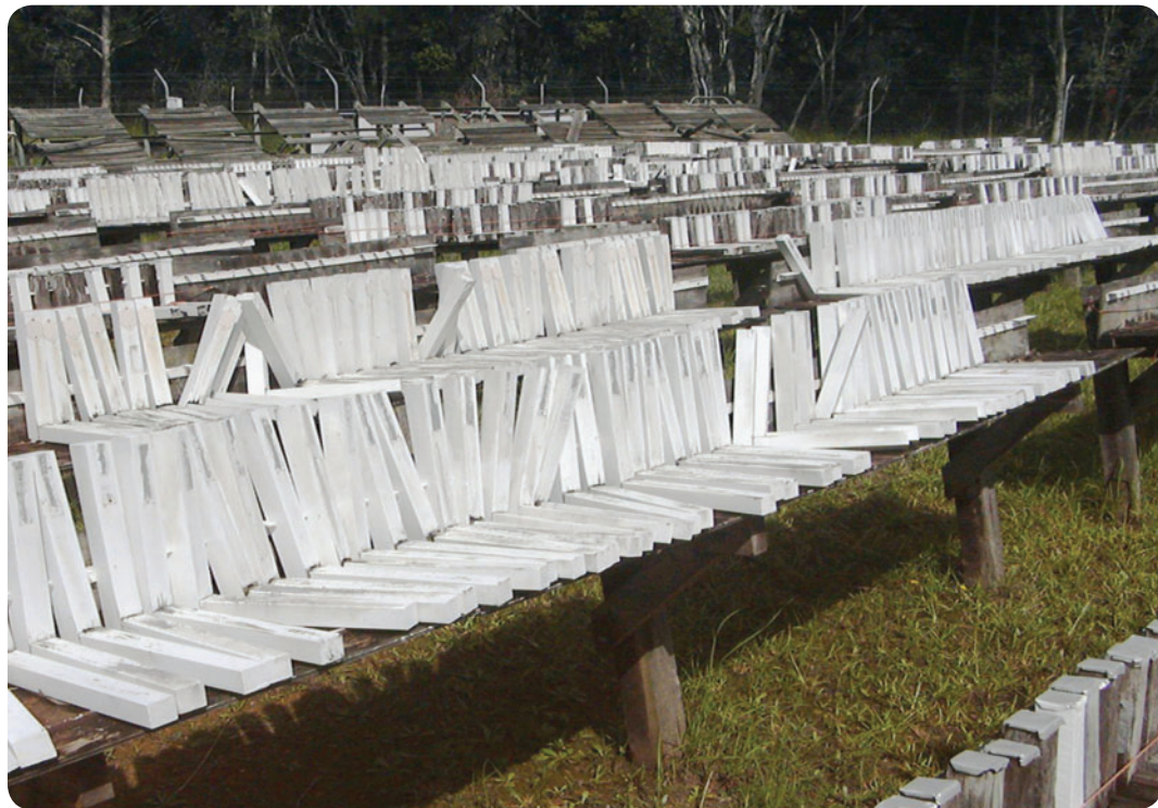
Above-ground durability test site in South-East Queensland.
