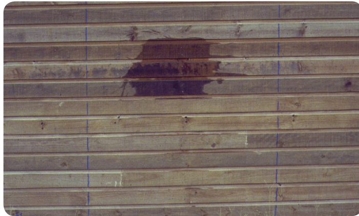
Bottom half of panel maintained with water repellent finish as indicated by 'water bucket' test.
